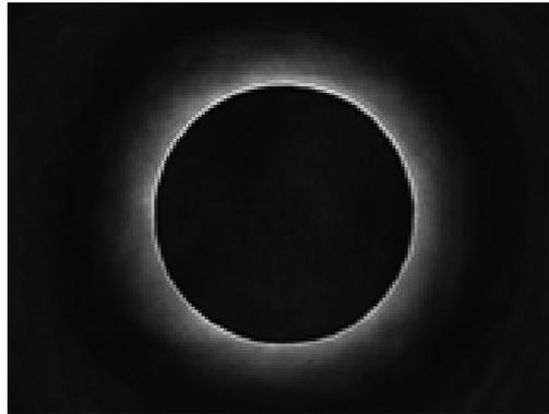
Figure 9. Output from a GPC-LS with the "darkness" phase mask installed
